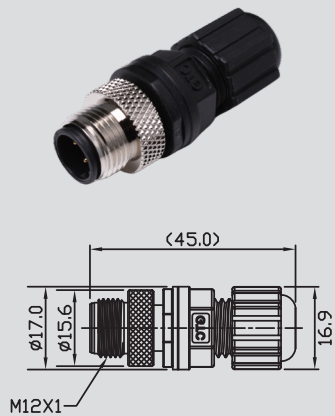
M12 D-Coding Field Installable Cable End Male Solder
