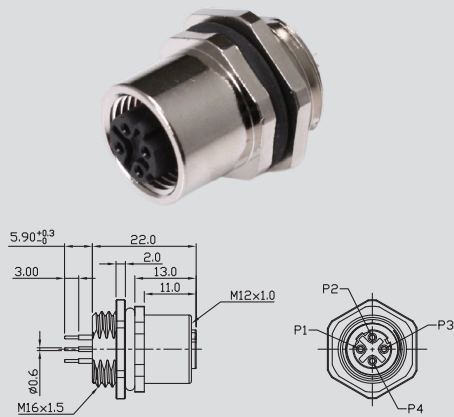
M12 D-Coding Panel Rear Mount Female Dip
