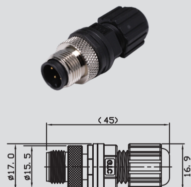
M12 A-Coding Field Installable Cable End Male Solder
