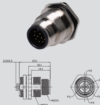
M12 A-Coding Panel Front/ Rear Mount Male Solder
