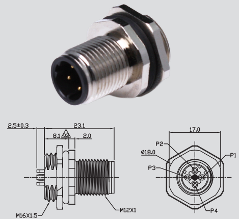
M12 D-Coding Panel Rear Mount Male Solder
