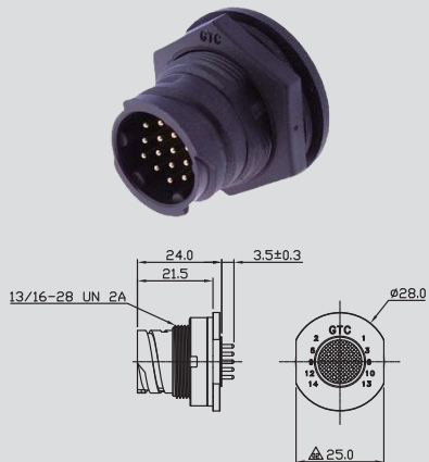
Plastic C3 Panel Male Solder Twist Lock
